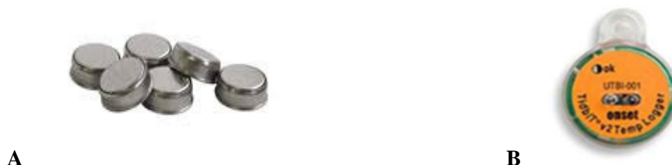
Figure 4. Temperature loggers A (I Button temperature logger (DS1922L/T) and B (Onset UTBI-001 Tidbit v2 temperature logger) installed at -25°C and 0-4°C
